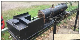
With the valve gear and cylinders refurbished attention now turned towards the cab and bunker. The tank had been sealed previously with a mix of filler and other sealants.
