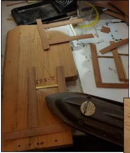
Here we have the other edge covered and also showing the tool used for ironing the veneer on. This iron is over 20 years old, from my days of R/C aircraft, this iron was used for covering wooden frames in 'Solartex or solarfilm' and was perfect for this particular job, I set the temp for 300c.
